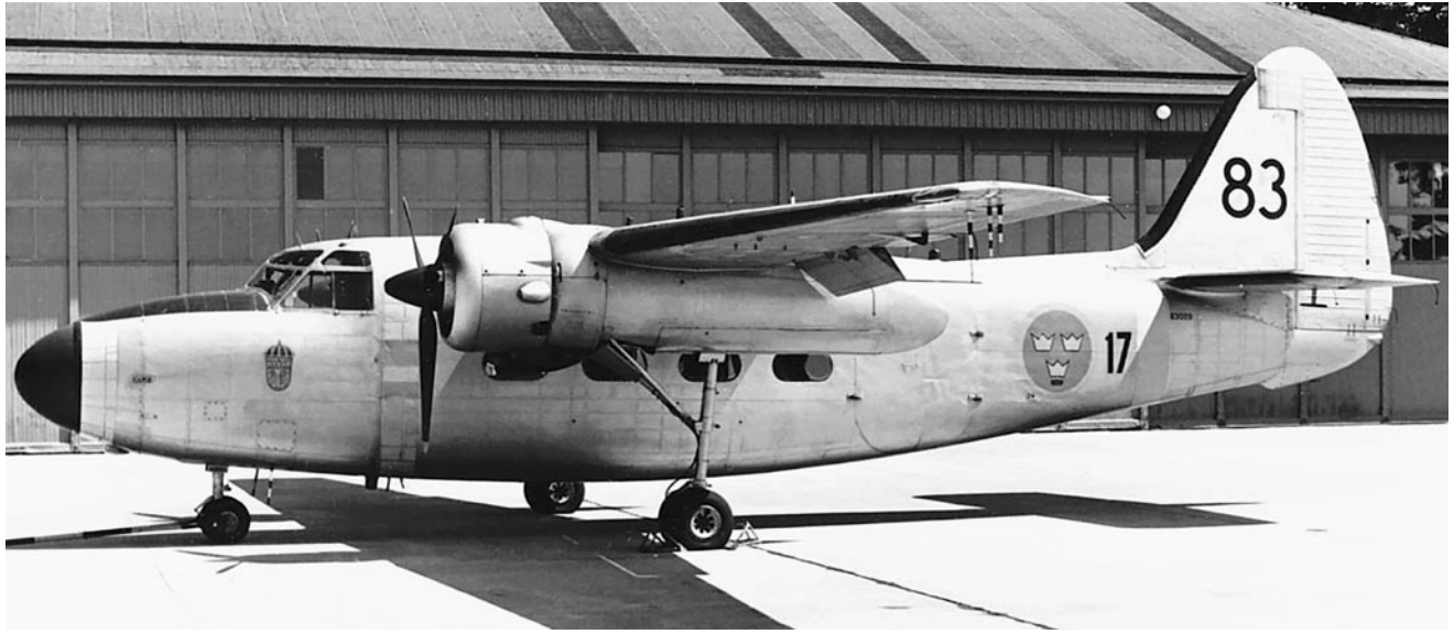
Above: An excellent picture of Tp 83 83009 of F 17. The photograph was possibly taken in the early 1960s. Note the Wing insignia on the forward fuselage and the faint dayglow markings on the front and rear fuselage (Arlanda Flygsamlingar Archives)
