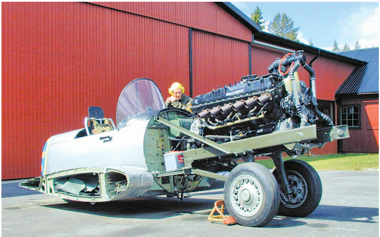
Below: The wing section of a Pembroke, powered by a Rolls-Royce Meteor engine (Merlin variant) from a Centurion tank, running on Saab Viggen wheels are the principal elements of this whimsical contraption built by Per Björkqvist – who works as a technician at Flygvapenmuseum – for the Jämtlands Flyg- och lottmuseum at Optand. The creator can be seen preparing to climb into the thing for an engine test (via Per Björkqvist)
