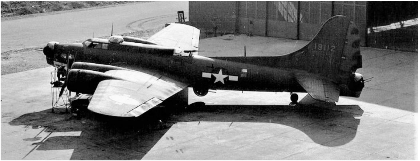
Image 3 shows the Dreamboat and lots of other B-17's the above is an enlargement of just the Dreamboat. The new nose, tail and upper turrets can be seen.
