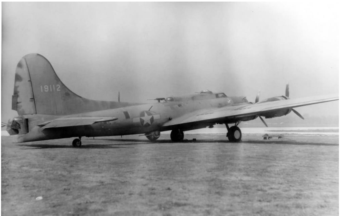
Image 6 In this picture the new second upper turret that replaces the two single waist gunners and the rear turret are seen.
