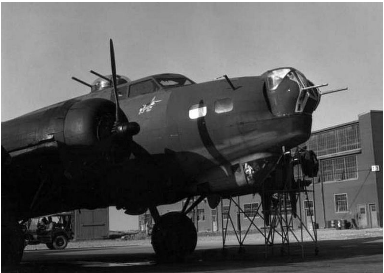
Image 4 shows the normal top turret and the new nose turret the bombardier/ navigators gondola can also be seen.
