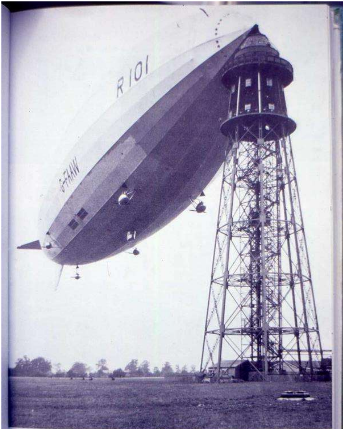
Ready for off – R.101C swings at the Cardington mast with the lift half-way between the ground and the boarding gallery just before dusk fell on the evening of 4th October 1930. All five engines are ready to start and fuel and stores are now all stowed – the 12 passengers and 42 crew members going aboard. [PLATE XXIII]
