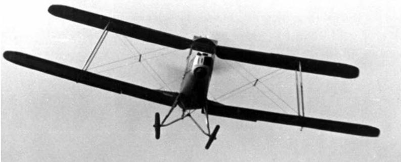
**Above:** The divided undercarriage hanging low when relieved of the aircraft's weight is made obvious in this fly-past photo. (RA Cole via JM Collection)
