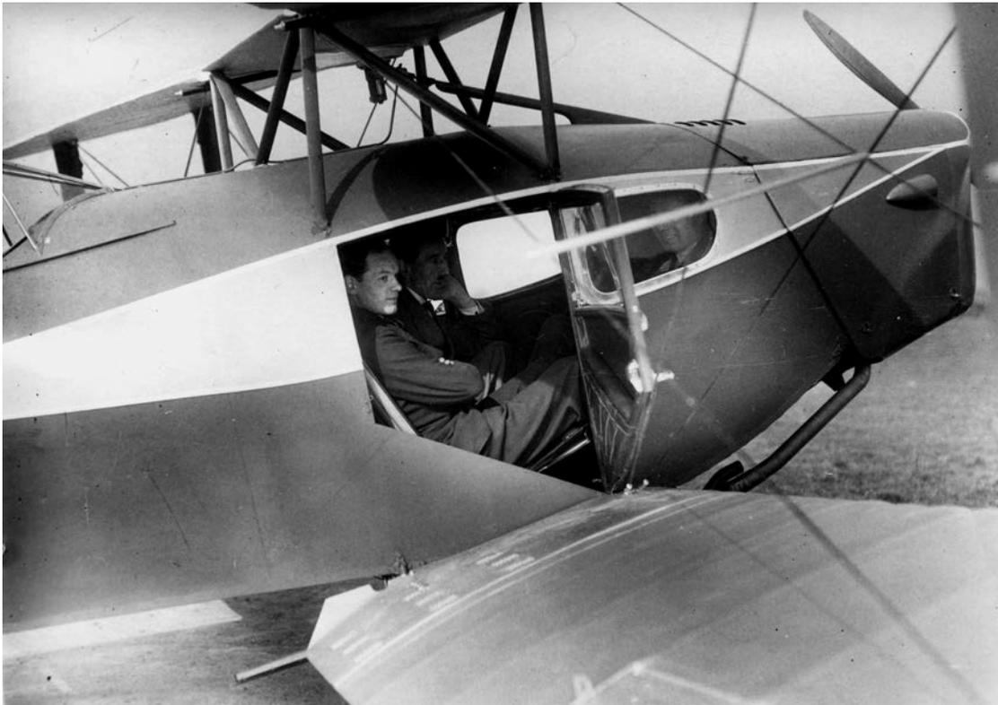
**Left:** Entry to the Fox Moth for passengers was over the low wing and accommodation consisted of a forward-facing bench seat for two and a rearward-facing bucket seat for one which was often replaced by another two-seat bench. The cabin occupants could be observed by the pilot by means of a large peephole on top of the instrument panel!
