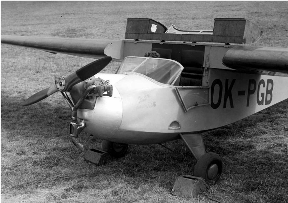
**Left:** OK-PGB now fitted with a Y-shaped exhaust and with the cockpit canopy in the open position, wing root folded back and side-panels down. (via JM Collection)
