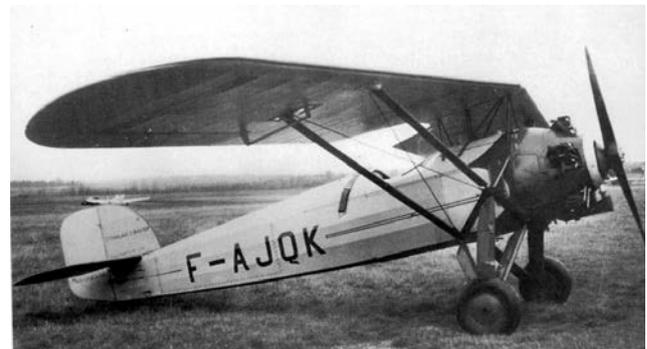
**Above:** F-AJQK was a single seat aerobatic parasol monoplane with a 60 hp Salmson radial, one of a batch of 14 registered to Cie Française d'Aviation in July 1930. (via JM Collection)
