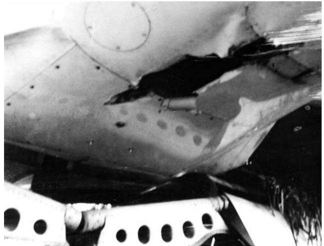
**Above:** Shrapnel damage to the fuselage underside affected the aircraft's hydraulic systems.
