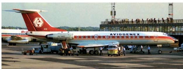
**Above:** The later model Tu-134s used by Aviogenex had a solid nose, no chin radar, and an elongated fairing on the elevators. YU-AHY was at Manchester on 7.6.82. (H John Black)
