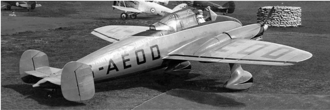
**Below:** G-AEOD shows off the tapered elliptical wing plan in this view. The rear cockpit gun position can also be seen although the aircraft was not armed at this time. The style of registration lettering makes the last two letters rather difficult to distinguish one from another. (Flight via JM Collection)
