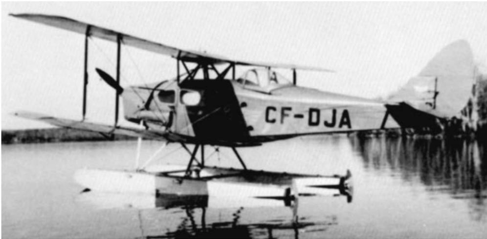
**Left:** C/n FM27 CF-DJA in a tranquil setting on an Ontario lake, fitted with Edo-2425 floats. (via JM Collection)
