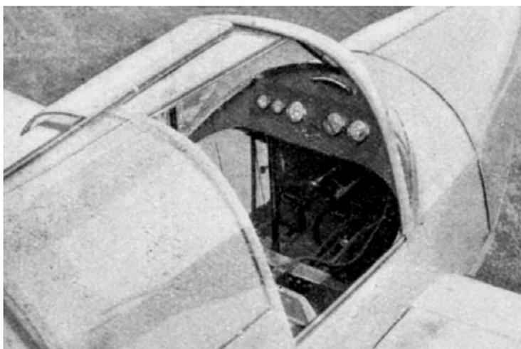
**Right:** The cockpit of the Knight was quite basic - but it was an experimental machine. From left to right the instruments were: oil pressure gauge, oil temperature, rpm, airspeed indication, and altimeter; above was a bubble level and below in the centre were the ignition switches and throttle knob. Dual controls were fitted. The two-piece sliding canopy is clearly seen. (via JM Collection)
