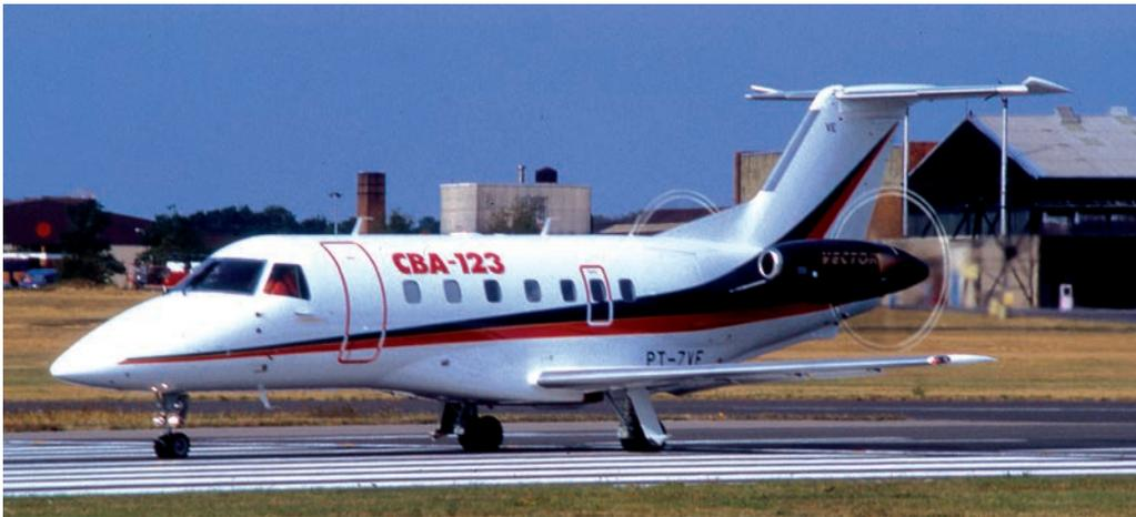
**Left:** The CBA-123 Vector prototype c/n 123801 PT-ZVE about to demonstrate at Farnborough on 2.9.90. The 19-seat regional airliner had many advanced features and was powered by two rear-mounted Garrett turboprops fitted with 6-blade pusher propellers. The second prototype PT-ZVB was flown at Paris the following year but no further examples were completed.
