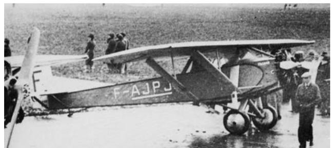
**Above:** F-AJPL was a Farman F.202 two or three-seat open cockpit light monoplane powered by a 120 hp Salmson 9 Ac radial.
