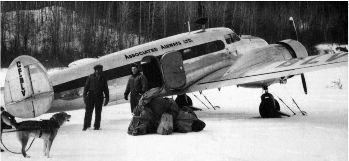
**Above:** CF-BLV was operated by Associated Airways in the early 1950s, here carrying supplies into the northland for further distribution by dog sled. Note the wheel/ski undercarriage used during the winter months. (via JM Collection)
