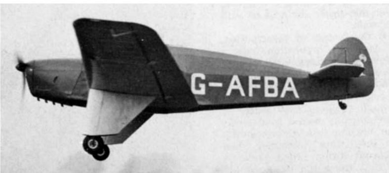
**Above:** The undercarriage fairings extend from just below the leading edge almost as far as the flaps. The four stub exhausts of the Cirrus Minor are now noticeable.
