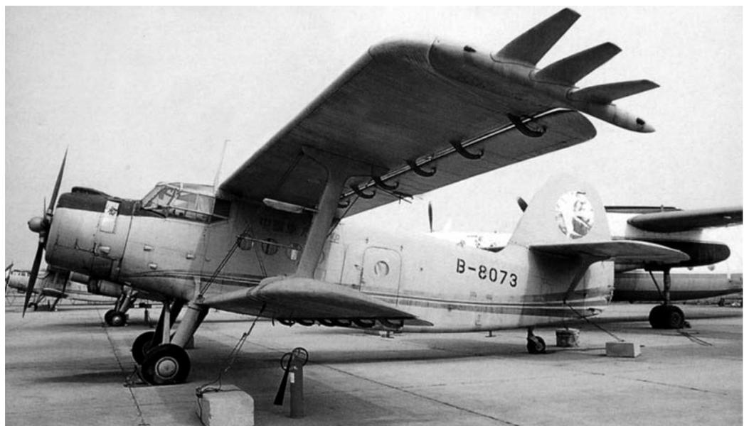
**Right:** An example of a Yunshuji Y-5, Chinese-built version of the Antonov An-2. B-8073 is in the somewhat weathered colours of China Eastern subsidiary Eastern General Aviation and was used for crop spraying. The feathered winglets are a modification to improve airflow and controllability. (via JM Collection)
