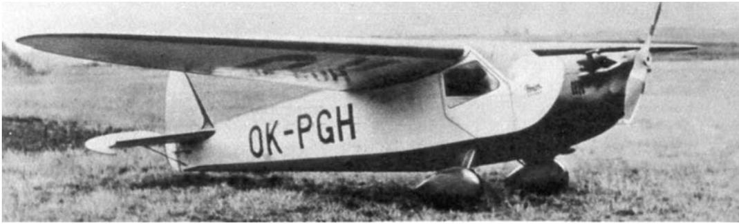
**Left:** The next stage in development was the E-117 which featured a fabric-covered steel tube fuselage and automobile-type entrance doors to the cockpit. The first prototype was OK-PGH as seen here. (via JM Collection)
