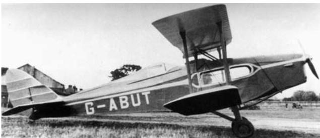
**Above:** Black and gold G-ABUT c/n 4002 was fitted with an enclosed cockpit, a Gipsy IIIA engine and had the fuel tank removed from the centre-section to the cabin to beat the handicappers and win the 1932 King's Cup at 124.25 mph flown by W L Hope.
