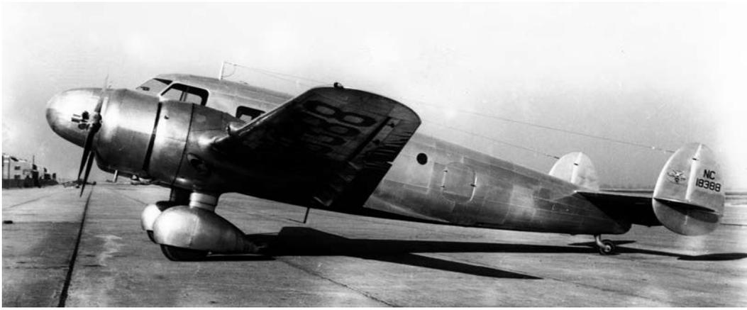
**Left:** This left-side view of the prototype, now registered NC18388, shows the door of the aft luggage compartment in the rear fuselage. The Barkley-Grow company logo is on the fin.
