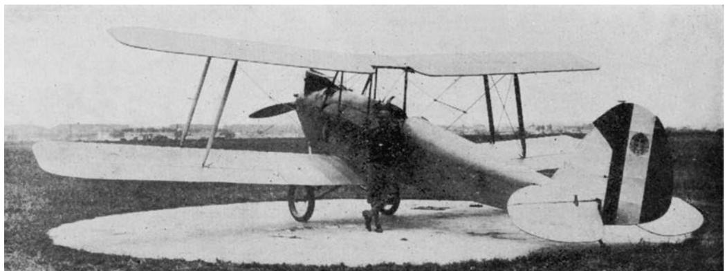
The wings were designed to fold to a maximum width of 3 metres to reduce storage space and on production aircraft Handley Page slots were added to the leading edge of the upper wings. Fuel was carried mainly in the centre-section gravity tank of 89 litres capacity but there was also an auxiliary tank in the fuselage ahead of the front cockpit containing 36 litres which could be manually pumped to the gravity tank. The aerobatic version relied entirely on a 40 litre fuselage tank.
