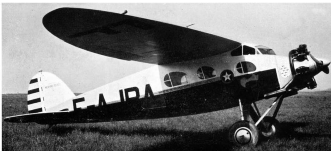
**Below:** Breguet 270 air observation post prototype F-AJRC shows the almost unlimited view for the observer in the rear cockpit. (via JM Collection)
