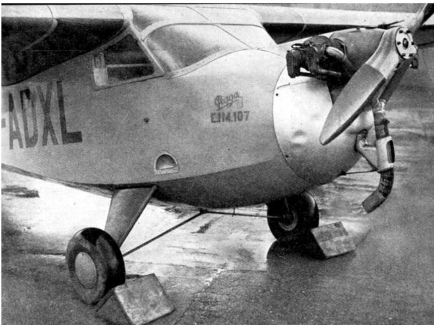
**Above:** Close-up of the UK demonstrator G-ADXL showing the exhaust with muffler fitted for cockpit heating, starboard side entry step and the type and c/n stencilled on the aircraft nose. (Flight via JM Collection)
