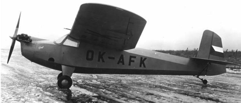
**Above and below:** This example of the Praga E-114 D was a post-war model, OK-AFK c/n 102. The hexagonal section fuselage shows up well in both views and also apparent is the redesigned fin and rudder shape. A tailwheel is fitted on this aircraft instead of the earlier tail-skid. (Both via JM Collection)
