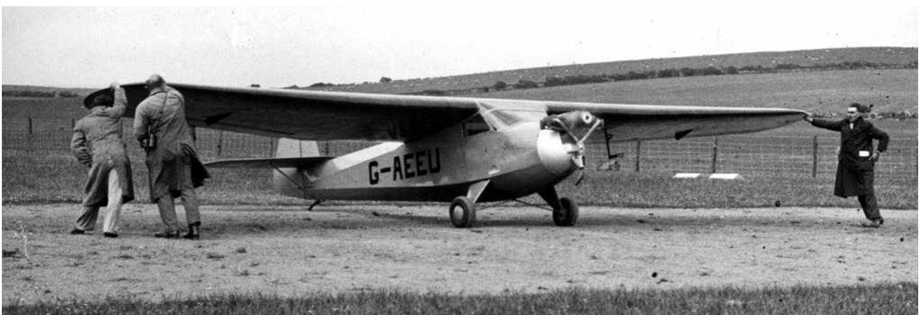
**Above:** G-AEEU was the second production Hillson Praga, c/n HA2, and the first on the UK Register. It is seen here being held back manually in the absence of brakes or chocks during an engine run before take-off. Having been stored during the war it was used as spares for G-AEUT in the 1950s, which coincidentally became the last airworthy Praga in the UK. (Aeroplane via JM Collection)
