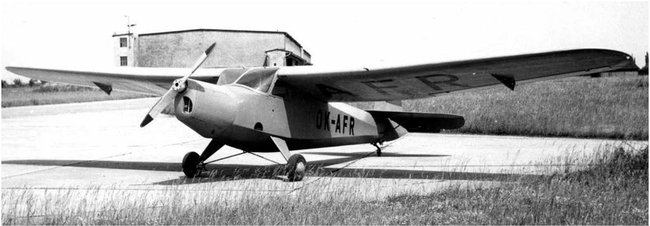
**Above:** Praga E-114M (65hp Walter Mikron III) OK-AFR c/n 109 shows the longer nose to accommodate the in-line engine and also a more marked dihedral of the outer wing sections. (via JM Collection)
