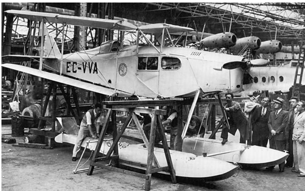
**Left:** C/n 4087 EC-VVA returned to the UK in late 1934 for conversion by Shorts at Rochester to a floatplane for an Amazon Expedition. With a Short Rangoon in the background the owners watch as the land wheels are removed prior to lowering the Fox Moth onto the floats.
