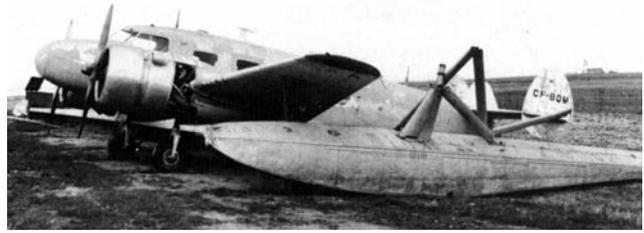
**Above:** Floatplane! The size of the EDO 65 floats is readily apparent in this view of CF-BQM back on its wheels and awaiting restoration at Calgary. The auxiliary central fin can just be seen. (via JM Collection)
