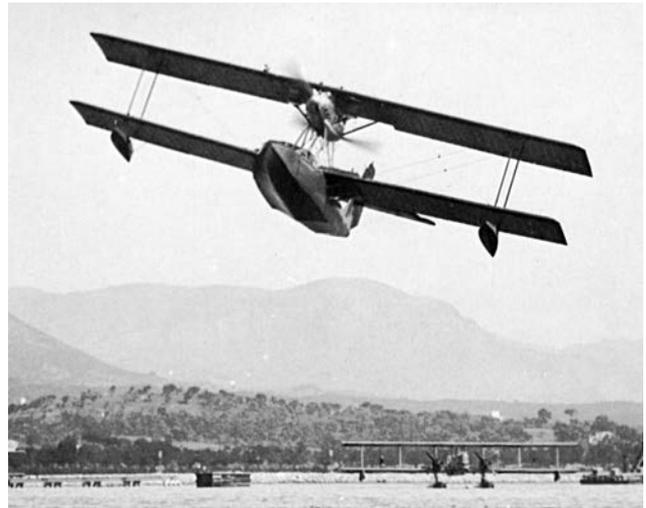
**Above:** F-AJIS, a CAMS 53-1 of Air Union seen departing from Ajaccio, Corsica, for Tunis. This model carried four passengers and a crew of two and was powered by a pair of back-to-back 500 hp Hispano-Suiza 12 Lbxr engines. (via JM Collection)
