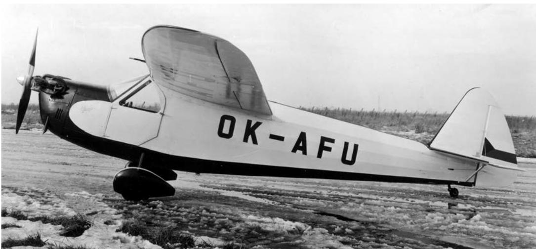
**Above and left:** The second prototype of the E-117 was c/n 2 OK-AFU. The shape of the doors has been modified and the rudder appears to have an increase in chord. Also visible is the revised pointed wing shape and the use of split flaps.
