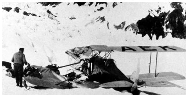
**Above:** ZK-AEK came to grief on the Franz Josef Glacier on 29.10.43 but was comprehensively rebuilt at Rongotai with a new fuselage.
