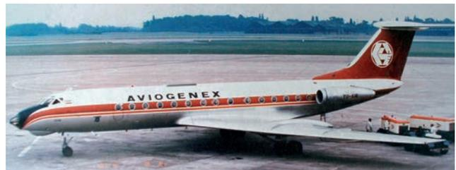
**Above:** YU-AHI "Zagreb" in the first Avioigenex colour scheme. The early Tu-134s used the transparent nose cone, chin radar and short strakes on the fuselage top. (Avioigenex via O Petrovic)
