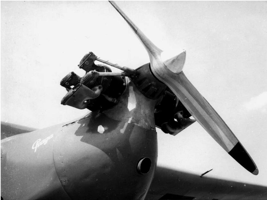
**Left:** The Praga D engine was a flat-four design which was intended to reduce drag, combining two cylinders into one housing on each side. The crankcase is aerodynamically shaped in order to fit cleanly into the forward part of the fuselage.
