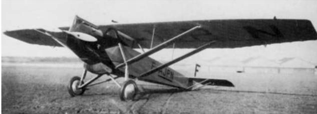
**Above:** F-AJPN was a F.201 and differed from the Salmson-powered F.200 and F.202 in having a 100 hp Hispano-Suiza 6Pa in-line engine and metal Ratier propeller. (via JM Collection)
