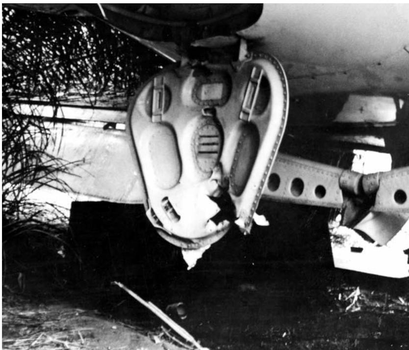
**Above:** The rear compartment - the "hell-hole" - of 5N-AER showing major damage. The proximity of palms is evidence that the 125 was pushed into a clearing on the edge of the airfield where repairs were to be carried out. (Michael I Draper Archive)
