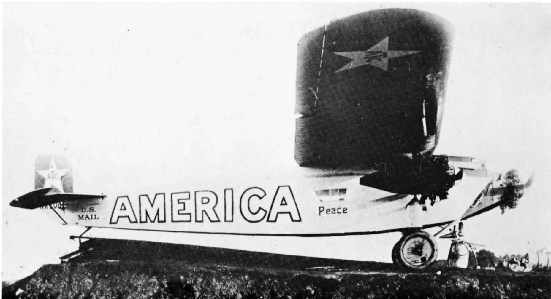
Above: Fokker C-2 NX-206 "America" (see entry for 16.4.27) standing on the ramp built to assist the take-off with the additional fuel load required for the Atlantic crossing attempt.
