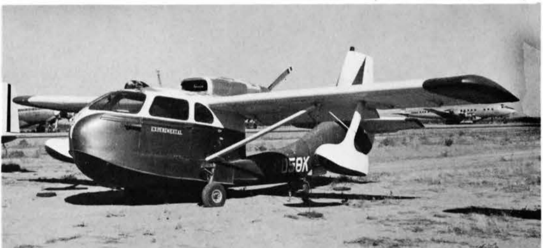
Non-standard Seabees. Above: N6291K, c/n 504, with large end-plates fitted to the wing tips at Opa Locka, 4.10.77. Below: N6058K, c/n 233 at Buckeye, Arizona 13.10.78 is marked 'experimental' and clearly has had its original Franklin substituted by a sleeker power unit. (both Ian MacFarlane)
