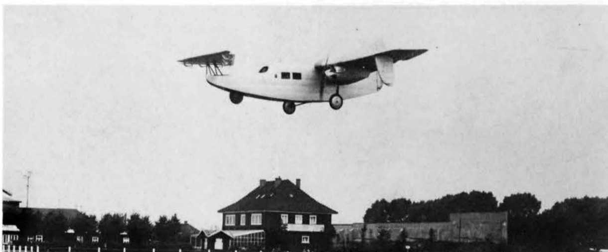
Right: The Focke-Wulf Ente on a test flight at Bremen (see 29.9.27). The name 'ente' means 'duck' and was of course an apt choice for an aircraft of canard wing layout.
