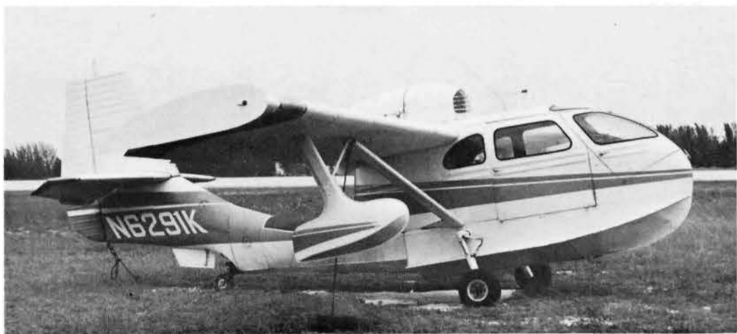
Non-standard Seabees. Above: N6291K, c/n 504, with large end-plates fitted to the wing tips at Opa Locka, 4.10.77. Below: N6058K, c/n 233 at Buckeye, Arizona 13.10.78 is marked 'experimental' and clearly has had its original Franklin substituted by a sleeker power unit. (both Ian MacFarlane)
