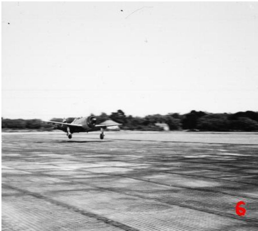
Image 5 shows the tented accomodation used by the 405th. Image 6 - A P47D landing on the Steel Matting Runway.
