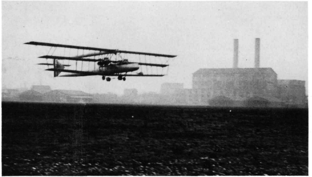
Above: The Monstre illustrated in AM.4/93 was a Voisin triplane and appeared in 1915 with four Salmson engines. It originally had no fin but the triangular one was fitted when it was modified to take 180 hp Hispano 8Ac engines in tandem pairs on the middle wing. It actually flew as witnessed by this photograph received via Jack Meaden. Is that the Issy power station in the background?
