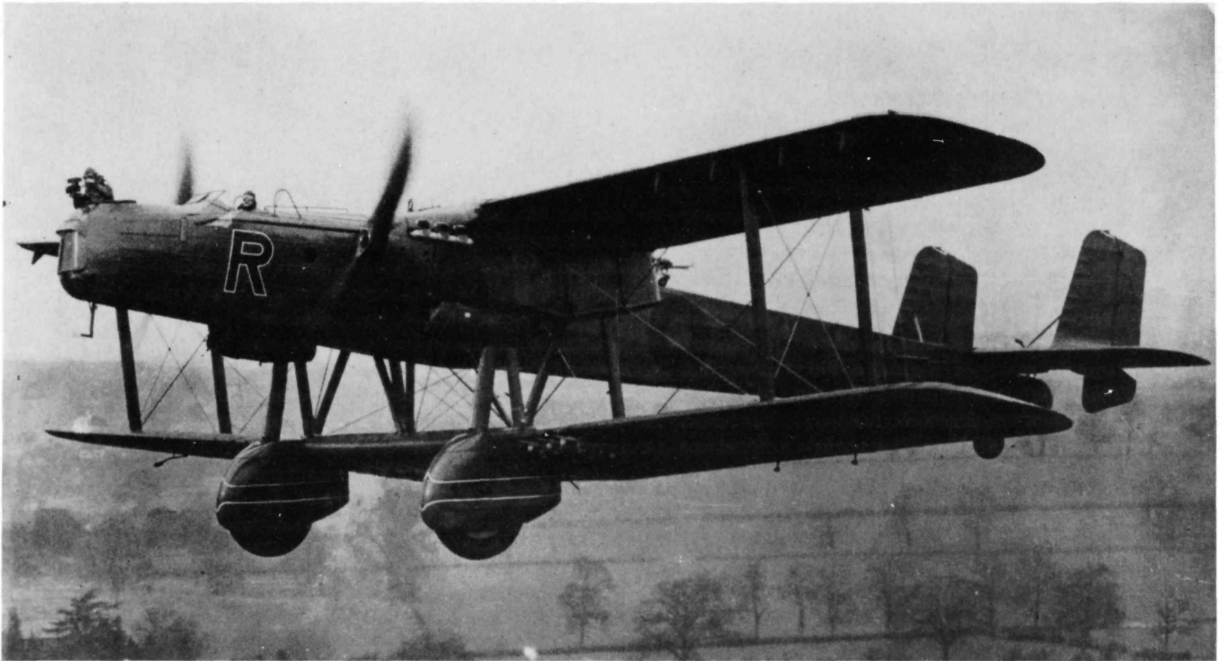
K3500, R of No.99 Squadron, with a cine-camera mounted in the nose. Note the propeller guards beside the cockpit
