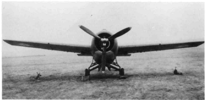
JV875 was used for testing the six rocket projectile mountings on the Wildcat VI
