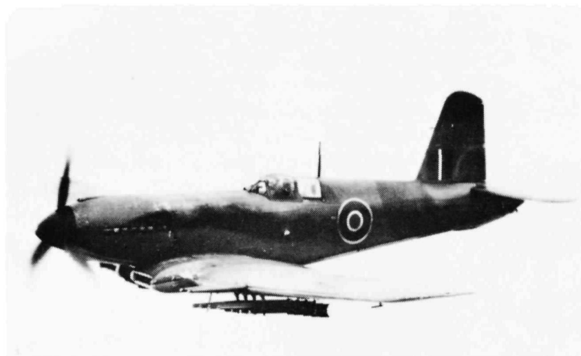
DK367 testing rocket projectiles at A&AEE
