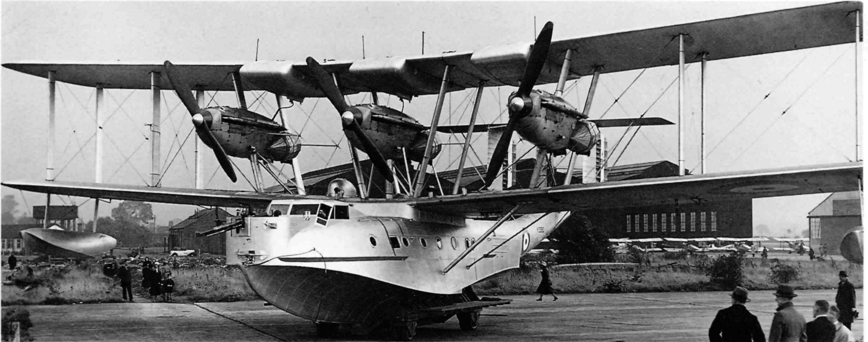
Perth K3580 on the ramp at Brough on October 1933 with Blackburn B.2s in the background. The 37 mm COW gun is fitted in the bows and the anchor is neatly stowed below it
