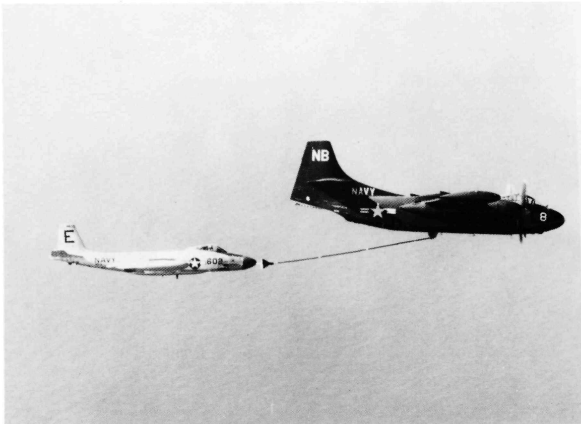
An AJ-2 of Port Lyautey-based VC-5 refuelling a F2H-4 of VC-4 det 34, assigned to CVG-8 aboard Lake Champlain in the Mediterranean, January 1955. (National Archives)
