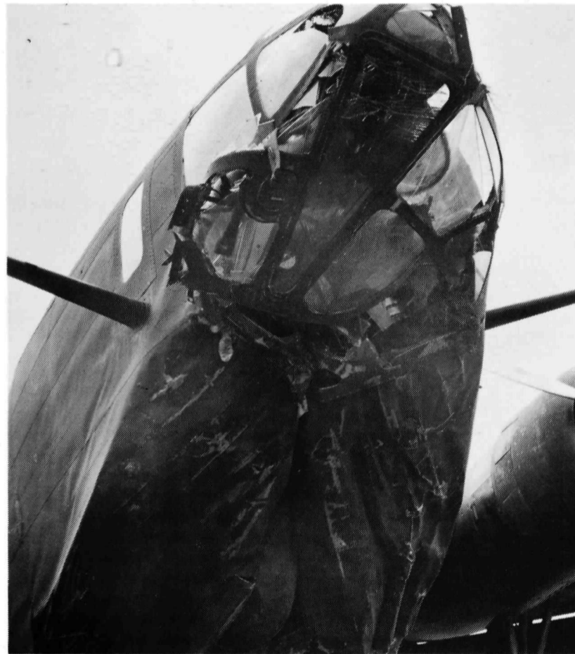
LIBERATOR NOSEWHEEL COLLAPSES
