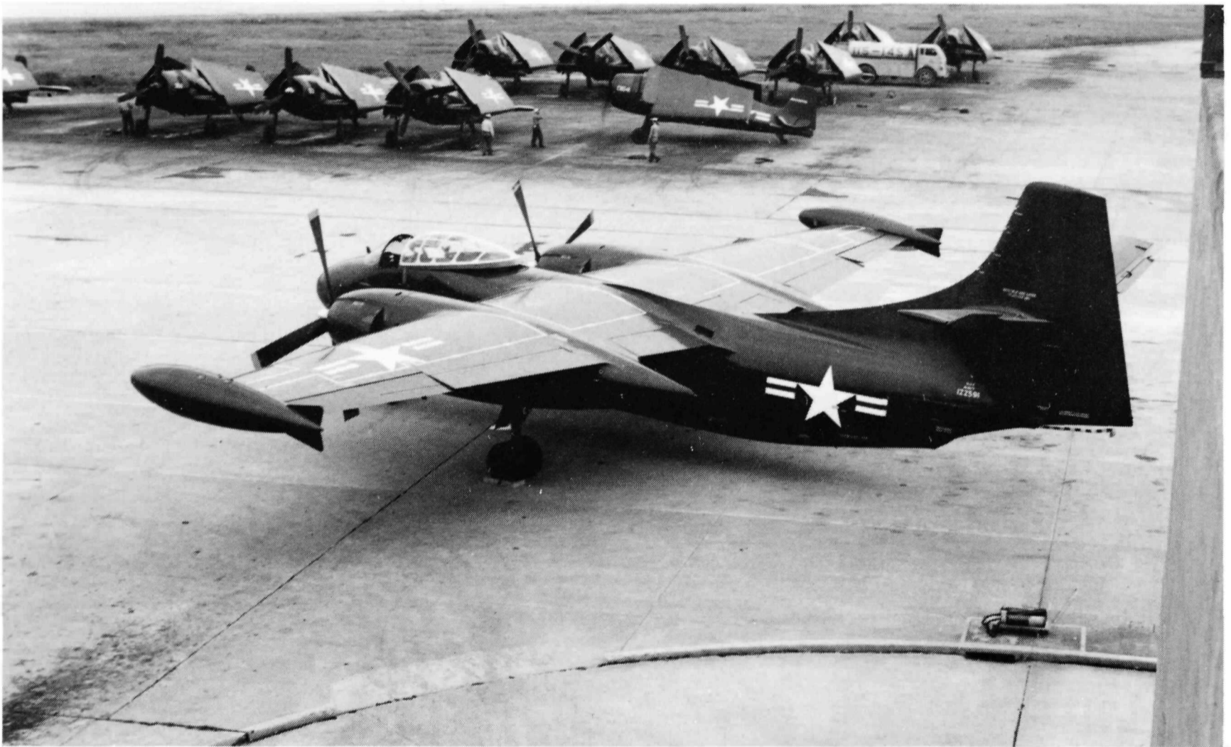
AJ-1 No.2 at NAS Anacostia in August 1949, just prior to delivery to VC-5. The fairing above the wing centre section housed the air intake for the jet engine. (National Archives)
