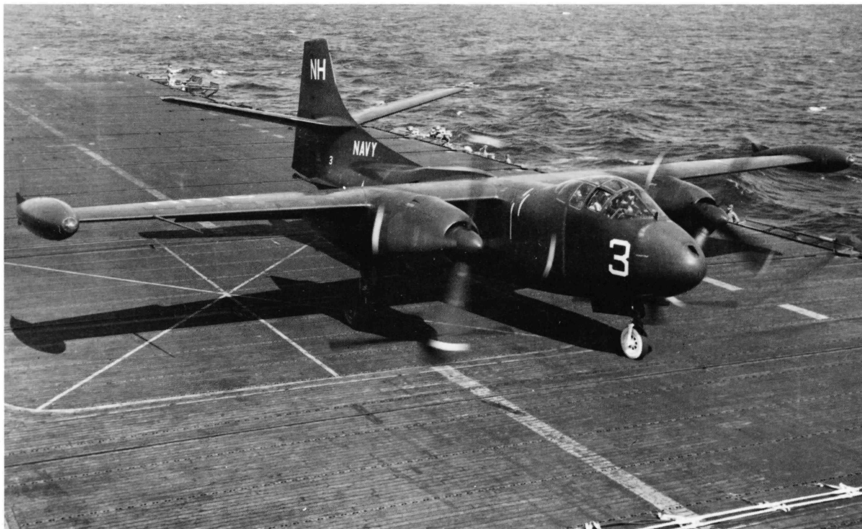
AJ-1 124165 of VC-7 aboard Wasp during a training cruise in February 1952. Not the dihedral on the tailplane. The AJ-2s had a taller fin and level tailplane; AJ-1s were later modified to this configuration. (National Archives)
