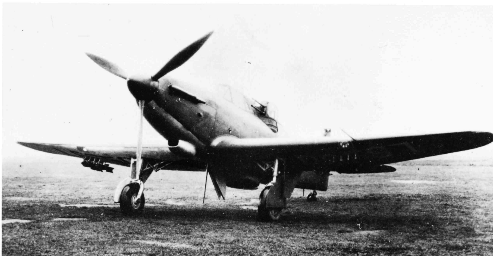
L6900 equipped with experimental bomb racks. (A&AEE)
