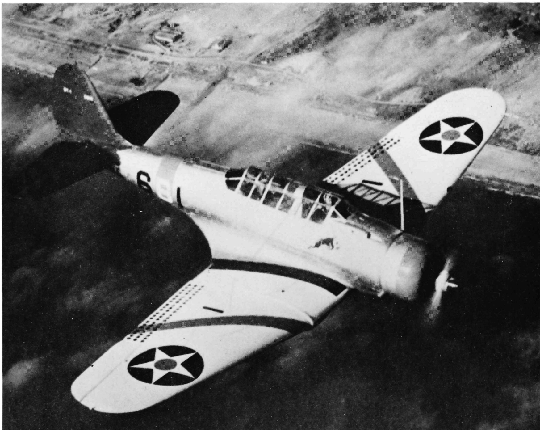
Another view of 0615. Note the circular perforations in the dive brakes. These produced a less disturbed air flow over the elevators than solid flaps. (Nat. Archives 80-G-463125)
