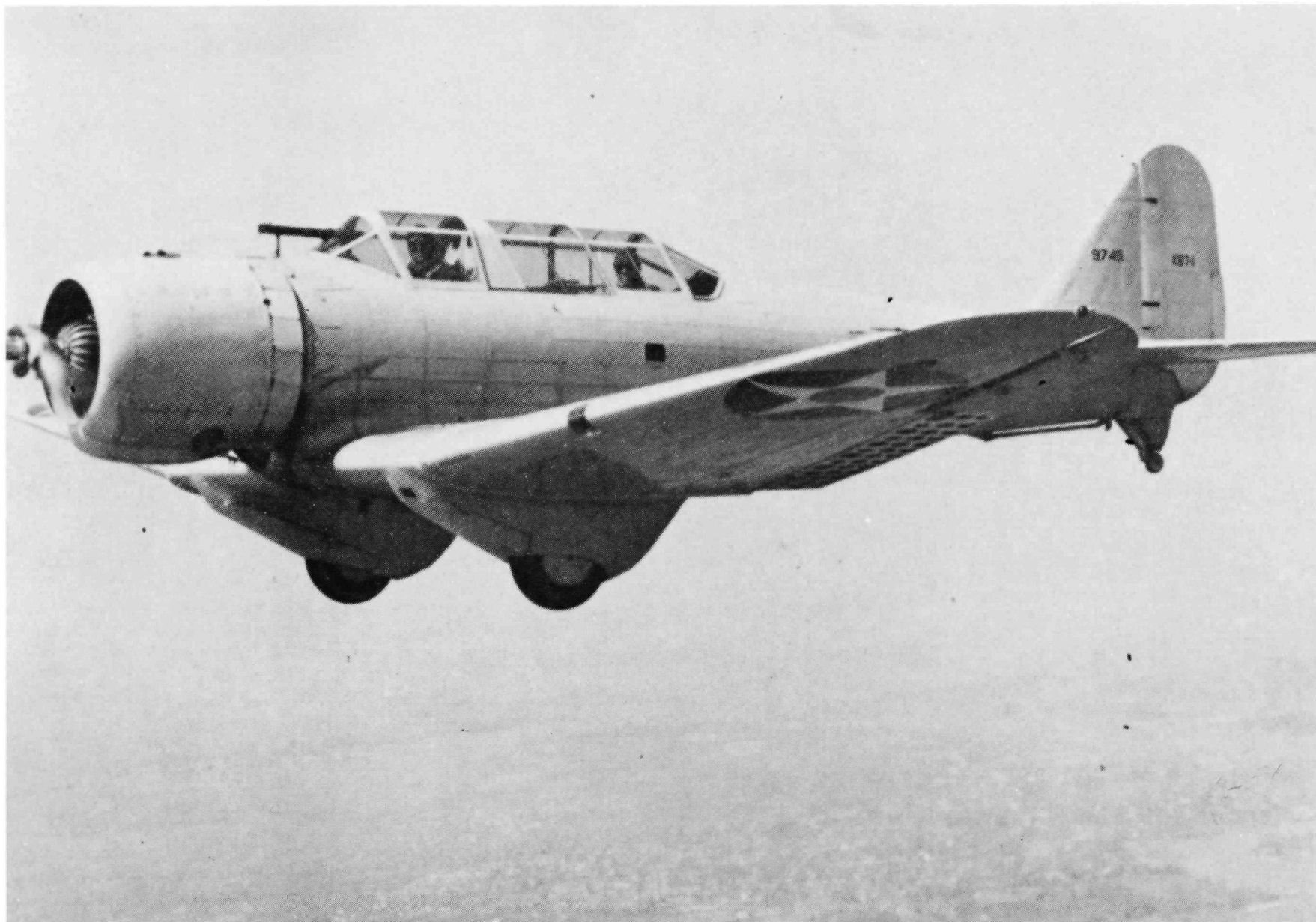
The prototype BT-1 shows off its distinctive semi-retractable undercarriage, April 1936 (Nat Archives 80-G-1053784)
