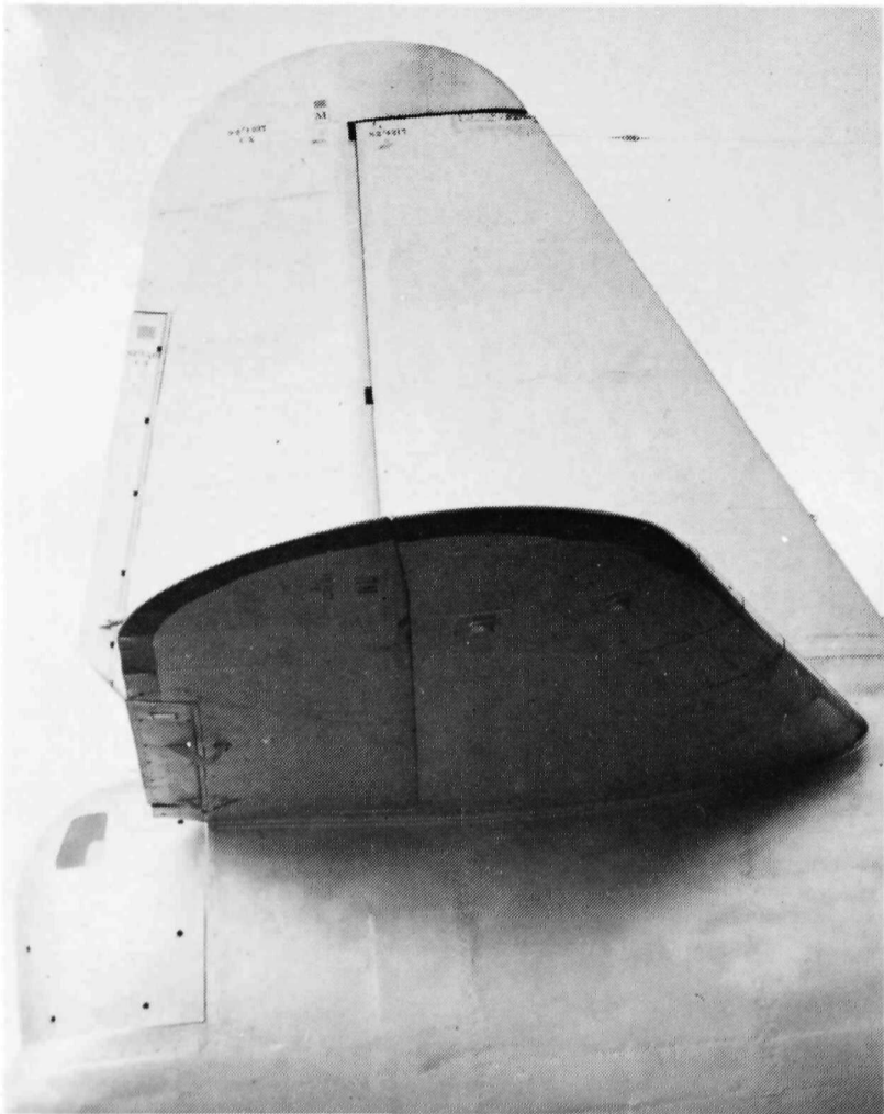
Above: Original and revised rudder shapes on L7248
