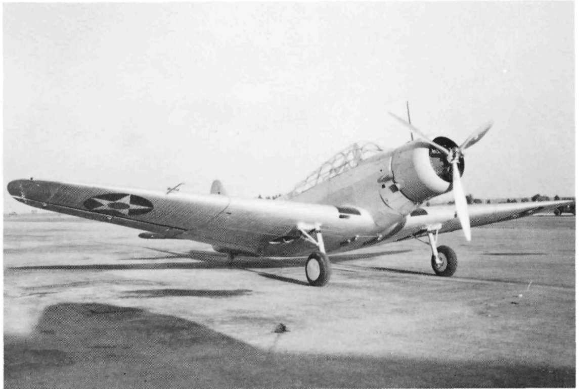
Prototype XTBD-1 in 1936 shows an earlier fin and rudder shape. In production version, fin was taller and rudder of narrower chord Nat Archives 72-AC-99D-4
