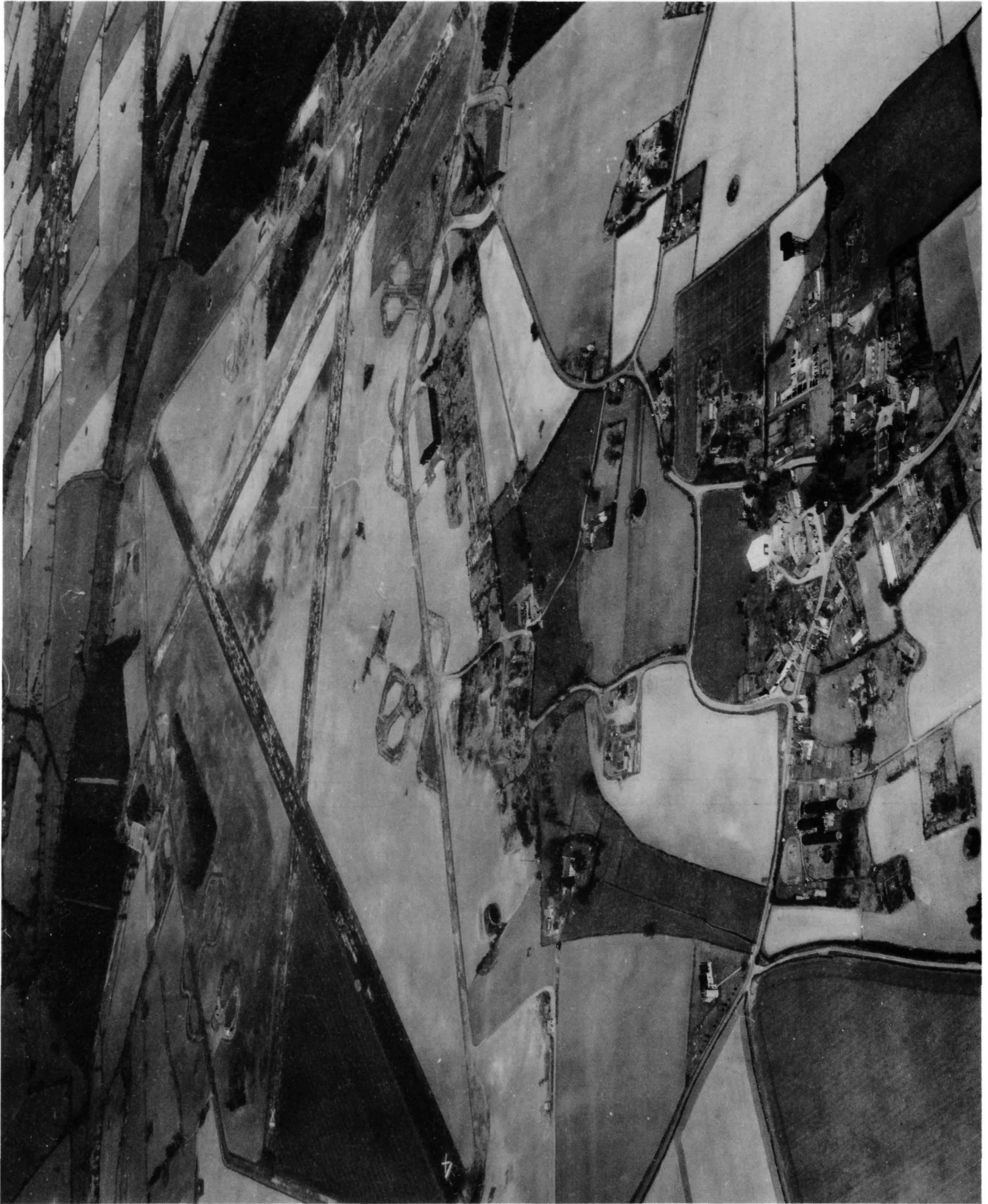
Little Snoring airfield facing north-east with Little Snoring village in the foreground. Photograph taken shortly after closure. Only one of the five main hangars remains. Two of the runways were 1,400 yds and one of 2,000 yds, 50 yds wide. The airfield's position was 3\frac{1}{2} miles NE of Fakenham at Latitude 52.21.38 North, 00.54.45 East.
