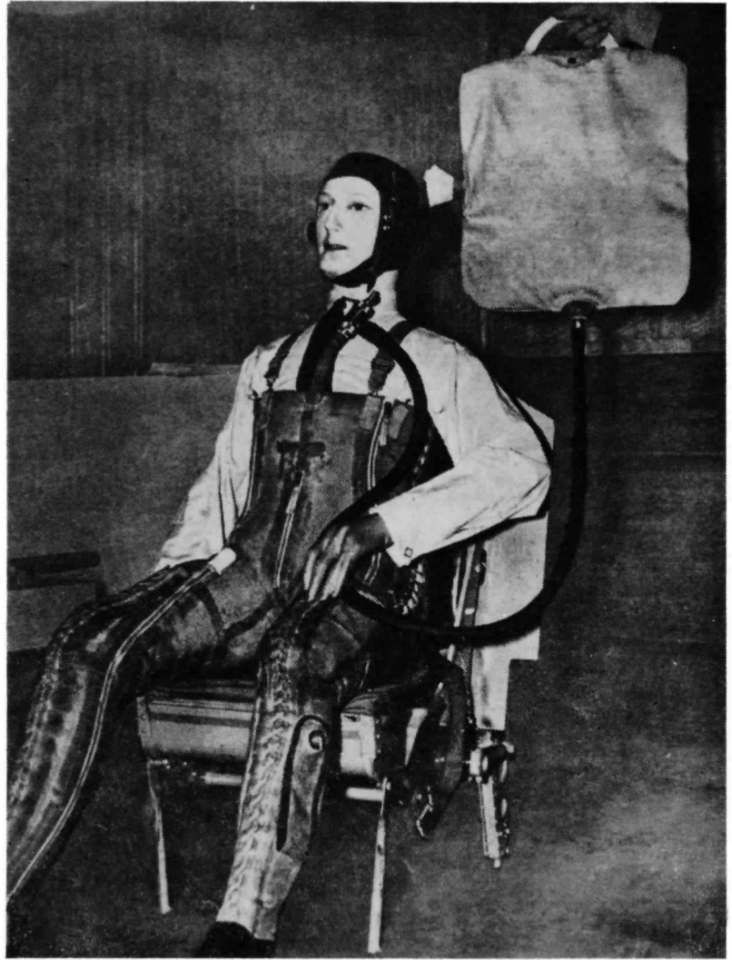
The Franks Suit fitted to a dummy
