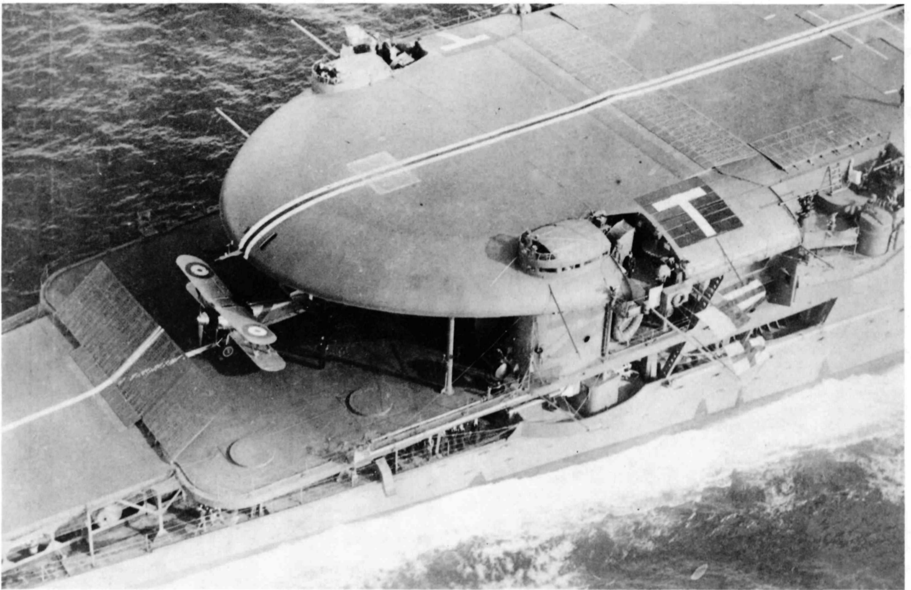
A Flycatcher parked behind the windbreak on the lower flying off deck. Note the exposed navigation and flying control positions which could trap an aircraft which swung on take-off (RAF Museum P.012724)
