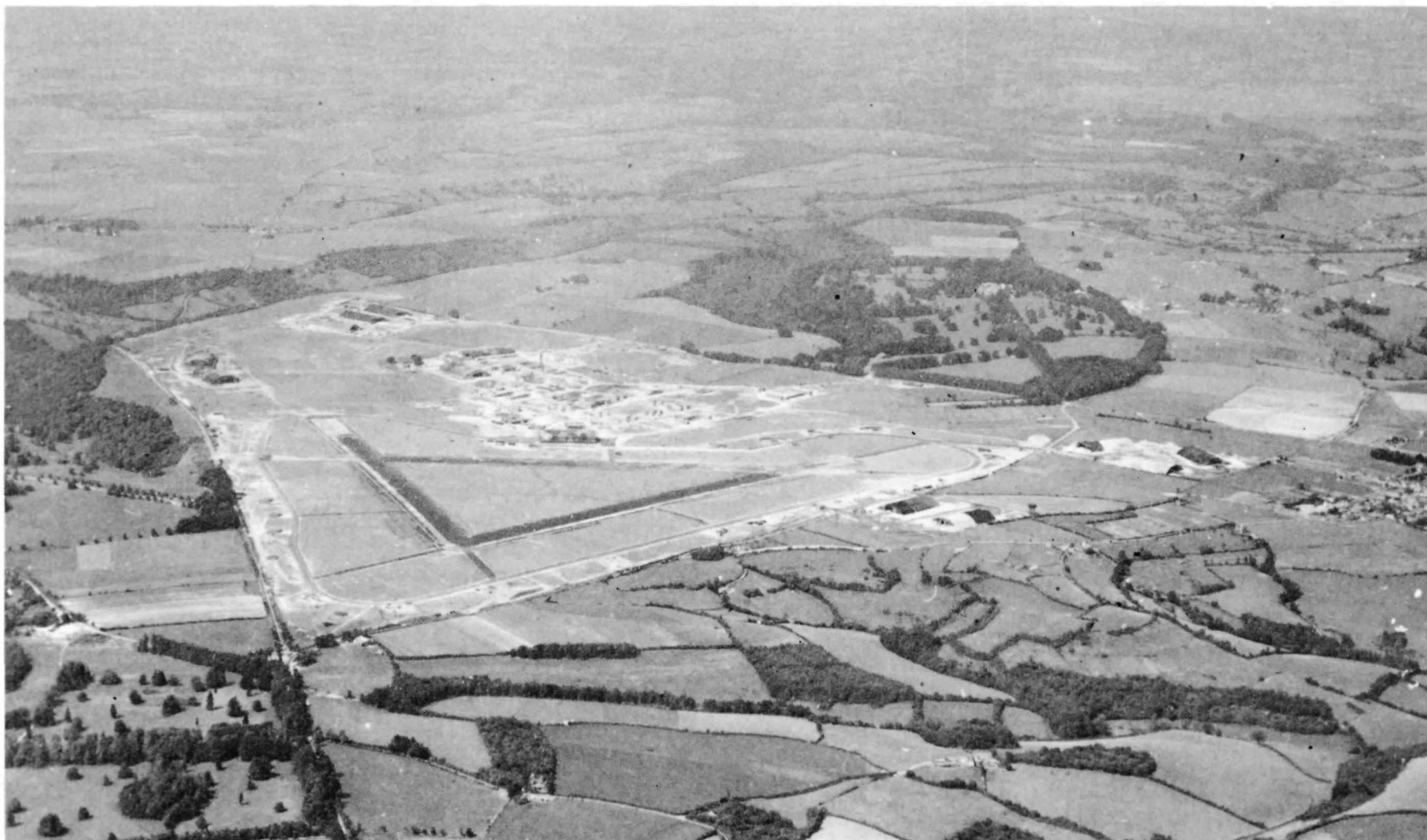
Colerne in June 1941, soon after completion of the runways. The hangar groups are widely dispersed. Running from south to north on the left of the photograph is the dead-straight Roman road, the Fosseway which bounded the airfield's west side. Later the runways were extended to join the perimeter track while the SW/NE runway was lengthened further. The fields to the north and east were used as dispersals for large numbers of stored aircraft both during and later the war.
