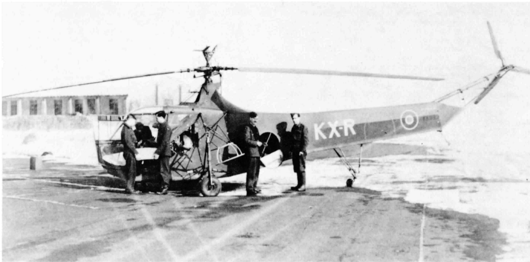
Hoverfly KK995 at Defford in 1947 on charge of the Telecommunications Flying Unit for radar response tests. It still carries its old 529 Squadron code 'KX-R' and is photographed while delivering supplies to the snowbound station. The side-mounted cage is part of the test installation (Ken Fry)
