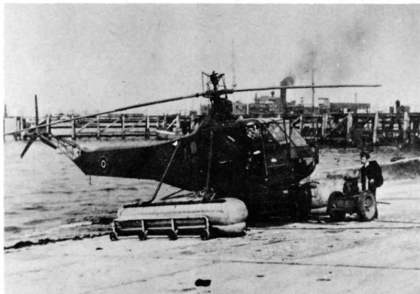
A float-equipped Hoverfly I operating from the hard in Portland Harbour (FAA Museum)
