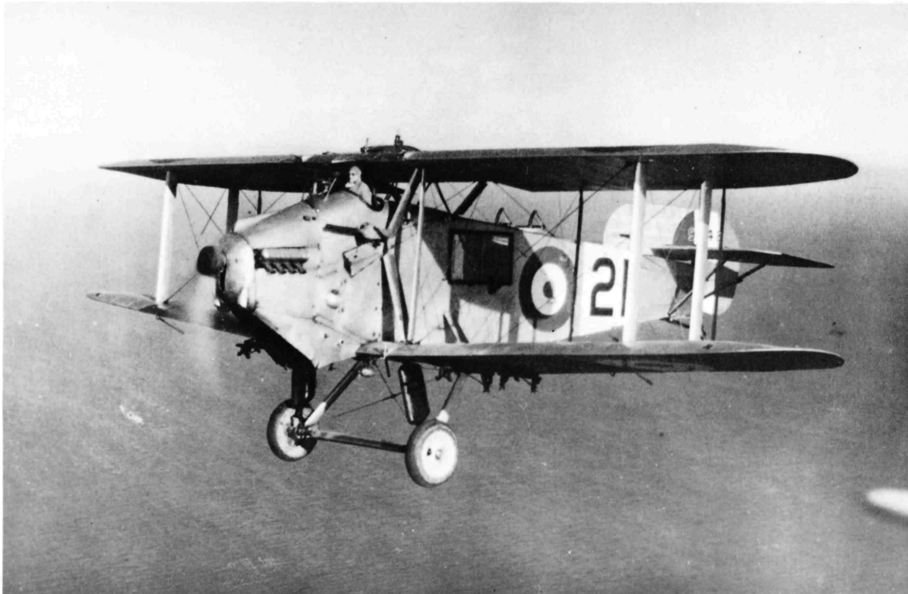
Bison II N9848, Fleet No.21, of No.423 Flight is fitted with a fixed Vickers gun for the pilot (RAF Museum P.2266)
