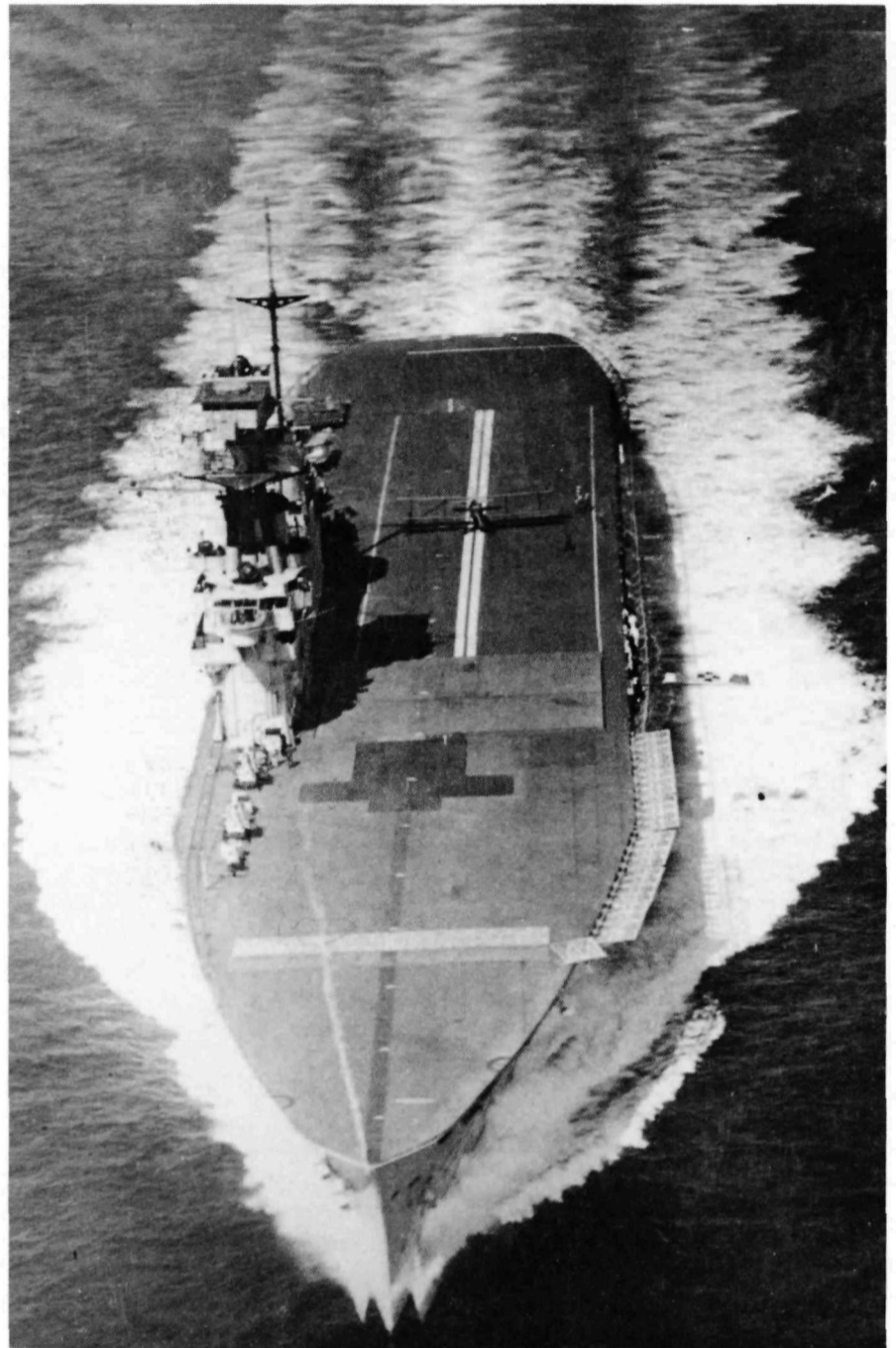
'Eagle' sailing not quite into wind with palisades down and a Fairey IIIIF on deck. Note the complex lift shape and the signalling mast over the port side (RAF Museum P.4264)
