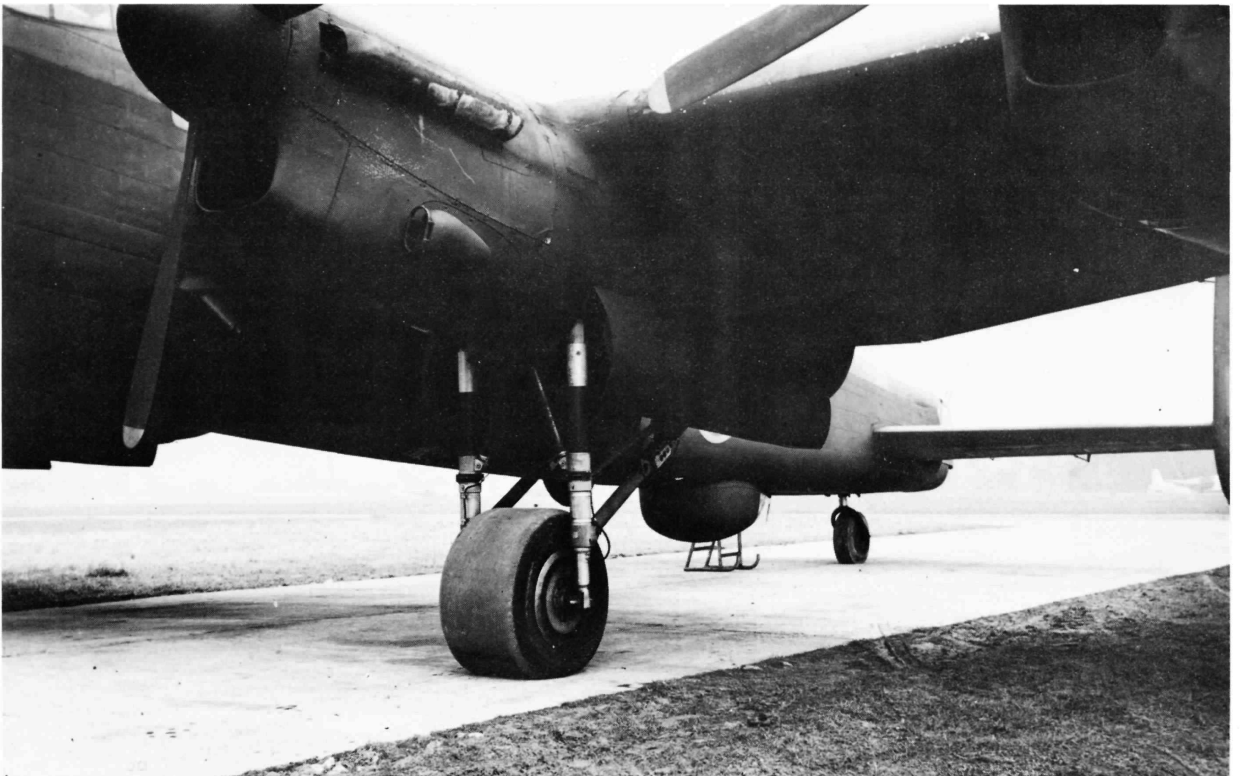
Above: The difference between a normal aero tyre and the new 'Compacta' tyre, both made by Dunlop, is clearly shown when the latter is fitted to the undercarriage of the Wellington
