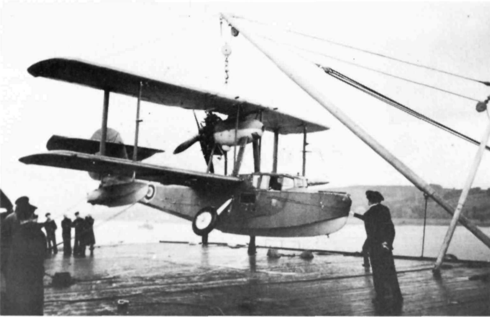
Emperor's Walrus was in frequent use for various tasks. Not being equipped with a seaplane crane, she had to rig a sheerlegs to hoist in the Shagbat
