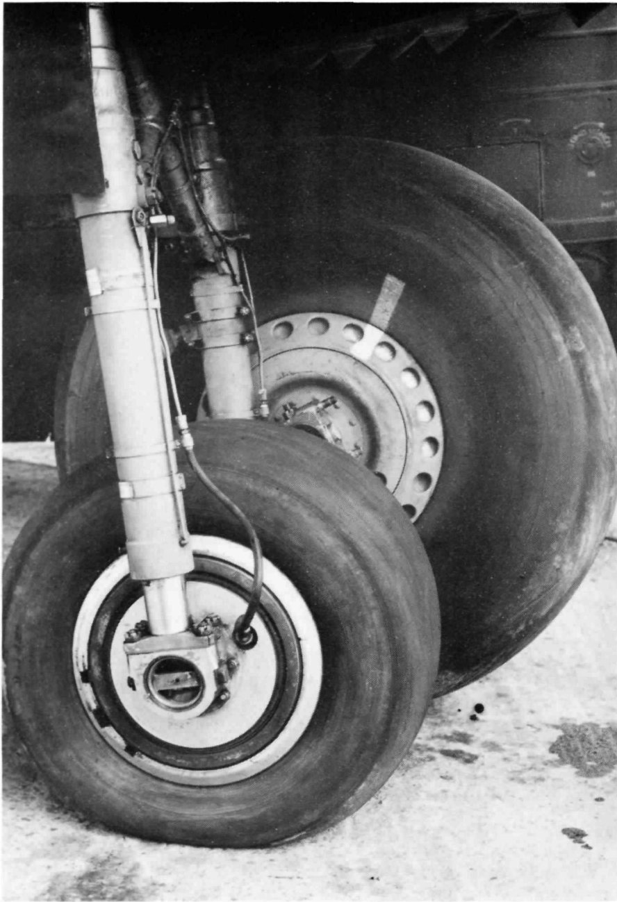
Above: The difference between a normal aero tyre and the new 'Compacta' tyre, both made by Dunlop, is clearly shown when the latter is fitted to the undercarriage of the Wellington
