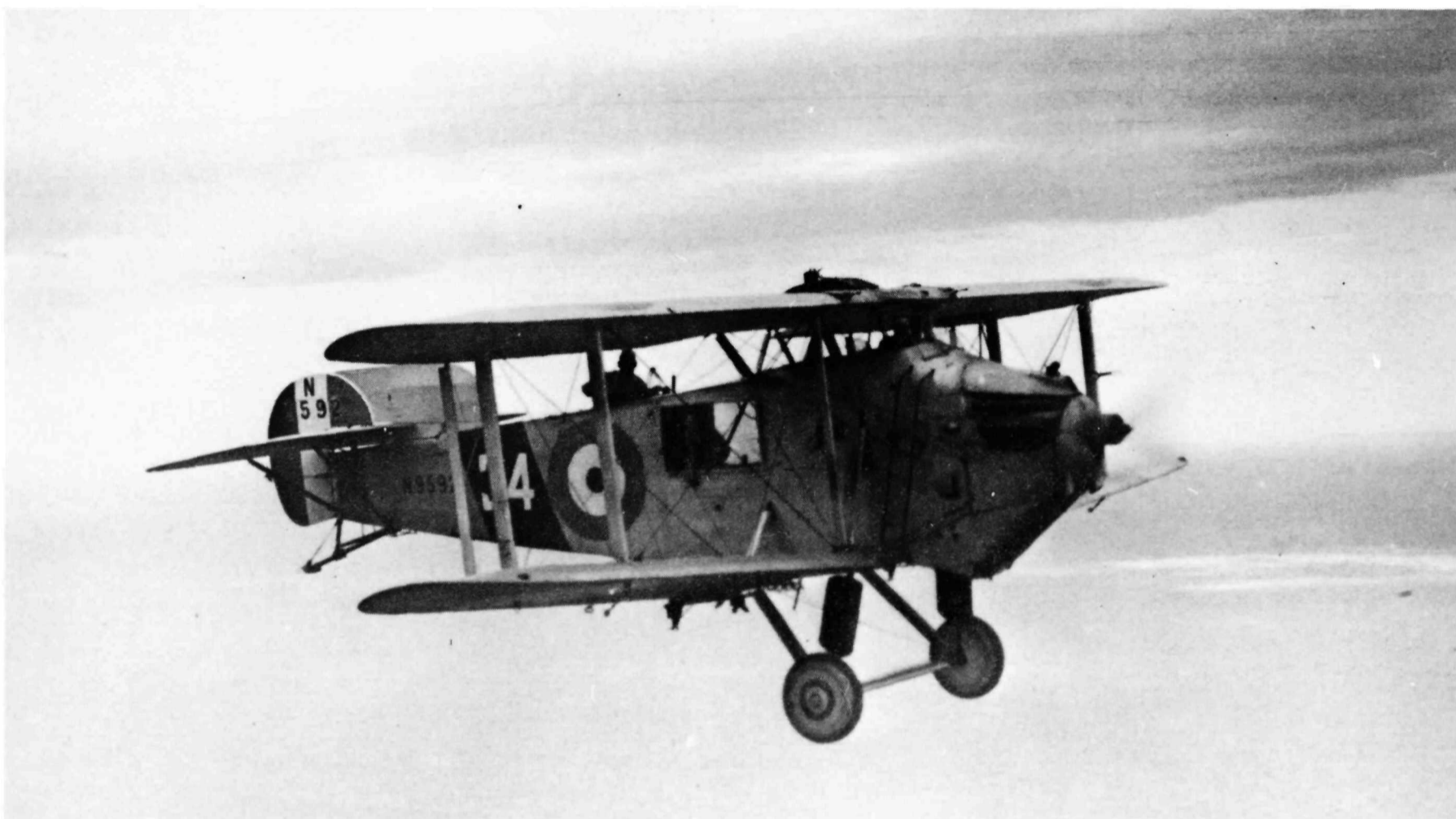
Bison N9592 of No.421B Flight carries 'Eagle's' fuselage band and Fleet Number '34'. Visible in this view are the bomb racks, the open window to the observer's cabin and the flight of steps providing access to the cockpit (RAF M P.2265)
