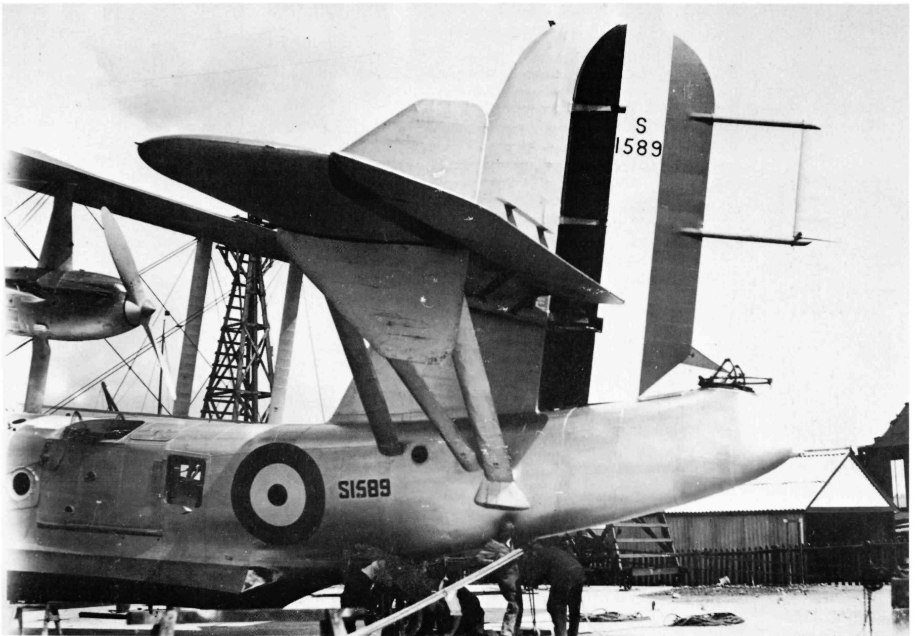
Below: The tail section showing the tail gun position and the servo-rudder (Short photo H 520D)
