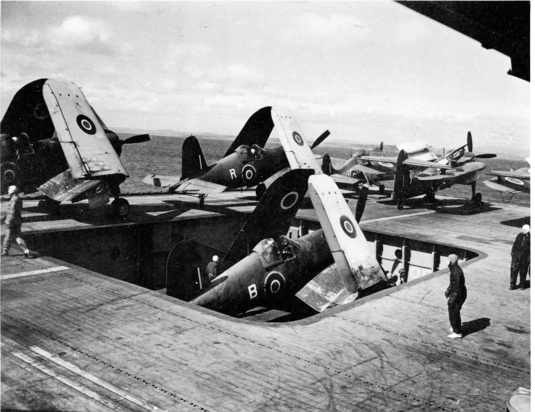
Taken in April 1945 during Smiter's deck landing training activities in the Firth of Forth, this view of the elevator area shows Corsairs, Barracudas and a Wildcat on deck. Note the cropped wingtips on the Corsairs to fit RN hangars.
