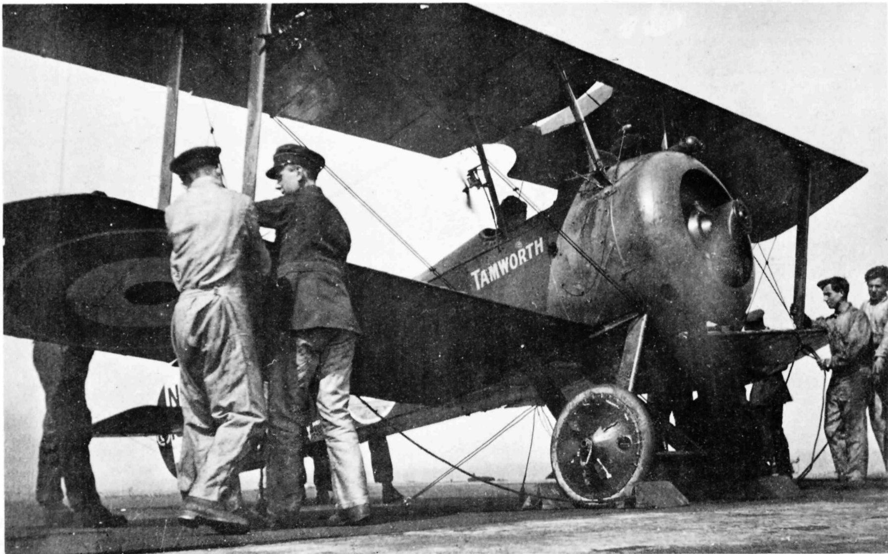
One of Argus Flight's Camels running up before take-off. Only the single Vickers gun is fitted. (IWM photo Q70162)
