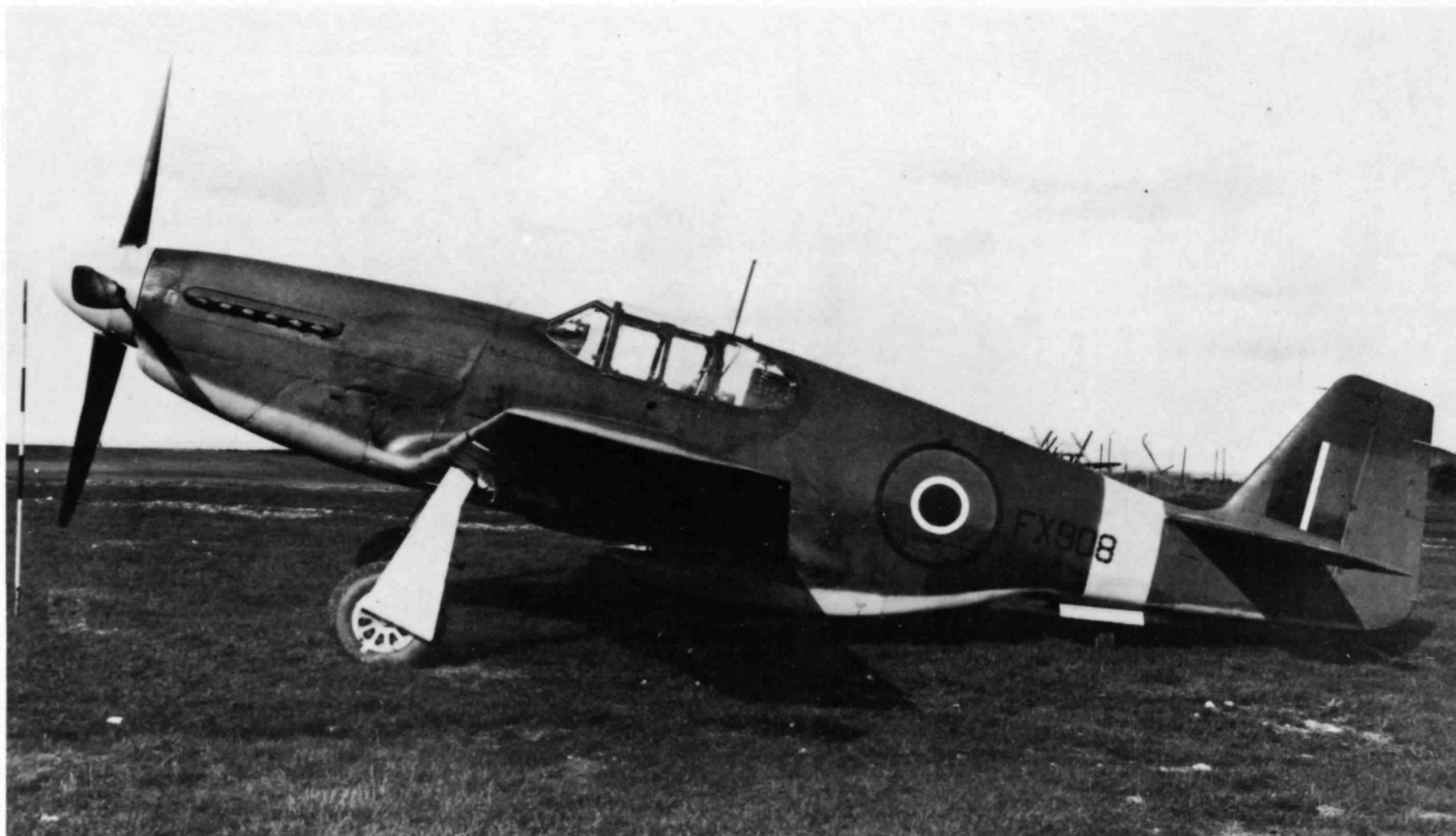
Mustang III FX908 (above) was photographed prior to delivery in October 1942 and illustrates well the lines of the original version of the Mustang III. The nose guns have disappeared and the air intake above the nose has been moved to under the nose fairing. The original cramped, flat-roofed canopy is retained with its sideways-opening exit but local modifications in Britain replaced many of these with bulged canopies as found on Spitfires. (RAF Museum photo P.5805)
