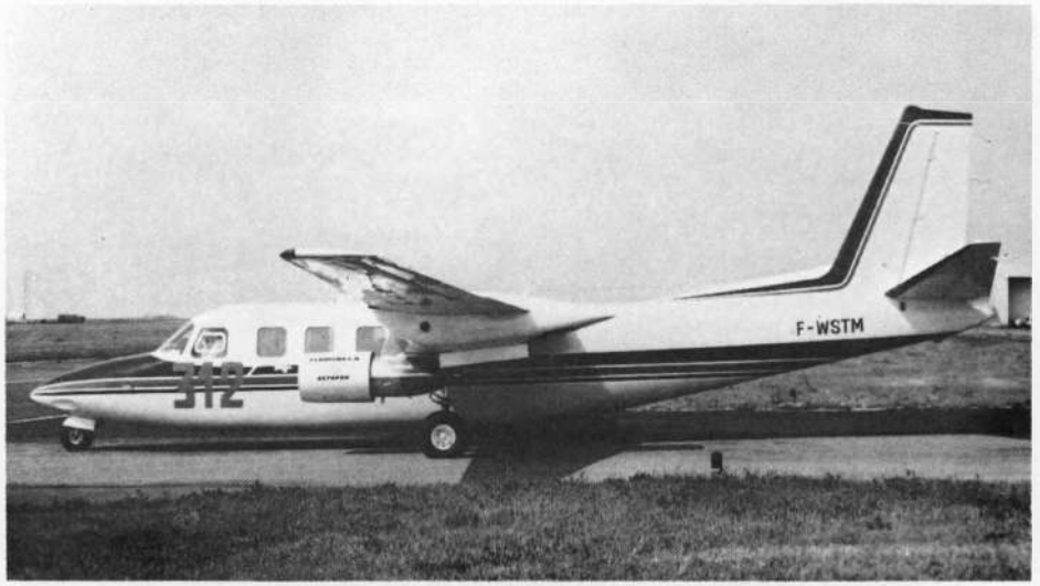
Aero Commander 680 VTU used by Turbomeca to test their Astafan IIA engines. Seen shortly after conversion to an engine testbed, in its original marks F-WSTM, it has been re-registered F-BSTM and is still in use at Pau (Photo: J.M.G. Gradidge)
