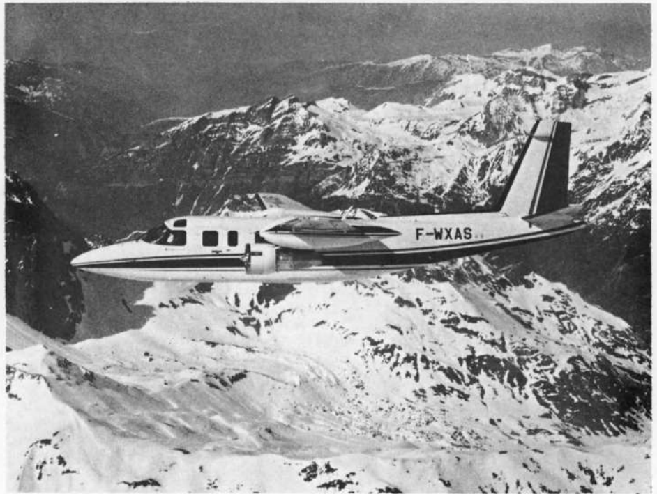
Turbomeca also have another conversion, Commander 690 ATU F-WXAS (since re-registered F-BXAS) which was adapted to test their Astafan IV-F 6 and Astafan IV G engines. The latter is a refined variant and powers the Fouga 90 twin-jet trainer (Photo: Turbomeca)
