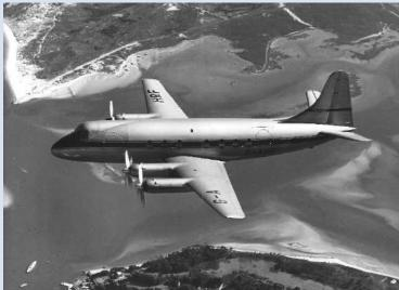
expected to have a still-air range of 1,725 miles at 20,000 feet with a cruising speed of 276 mph.
