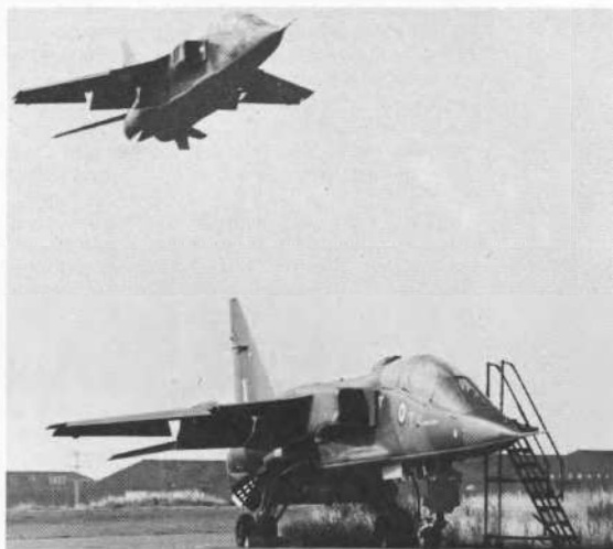
Above: EO2 (French serial C) flies slowly over BO8 (XW566), the first British two-seater also shown below. Note length of the nose compared with the single-seaters opposite.
