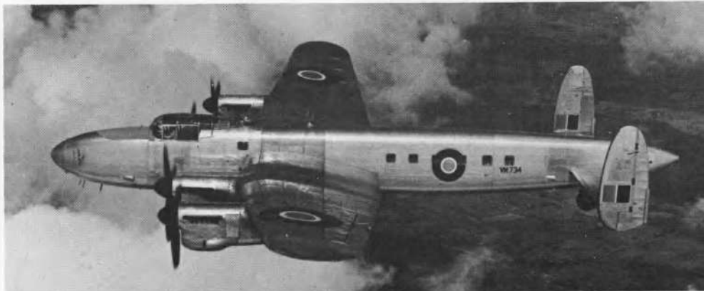
Above: Britain's earliest post-war long range transport was the Avro Lancrastrian, a civil conversion of the Lancaster bomber with faired in nose and rear fuselage. Illustrated is VM734. Below: Further
