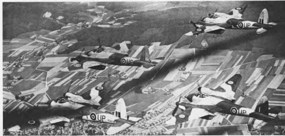
Above: Anson VP514 and Mosquito PR.34 RG245 carrying out mapping work over the London area in January 1949. Note the camera ports beneath the fuselages.
