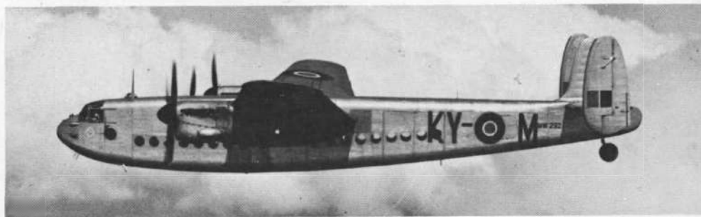
Above: Britain's earliest post-war long range transport was the Avro Lancrastrian, a civil conversion of the Lancaster bomber with faired in nose and rear fuselage. Illustrated is VM734. Below: Further
