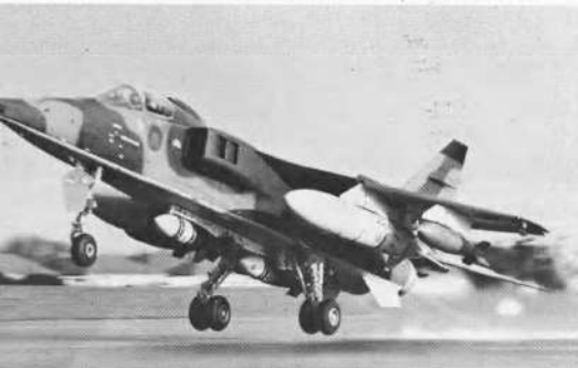
Above: Two production aircraft – S1 (XX108) with twin Matra rocket launchers and 1,200 litre fuel tank and S2 (XX109) with two 1,200 litre tanks and three 1,000 lb bombs. Below: SO7 (XW563) and SO6 (XW560).
