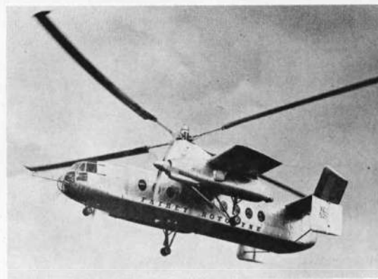
Top: Gyrodyne G-AIKF and below the Jet Gyrodyne XJ389 can be readily compared in these photographs. Right: The Rotodyne XE521 in an early configuration - note splayed out fins ( Flight photo 37176s).
