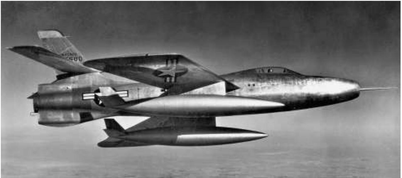
Above: A view of the prototype, 46-680 at altitude, carrying a pair of 541 US gallon external fuel tanks. The configuration of the rocket engine fairings suggest that these are vertically aligned with two rocket ports above and two below the jet pipe, as arranged for the XLR27 engine which was never fitted
