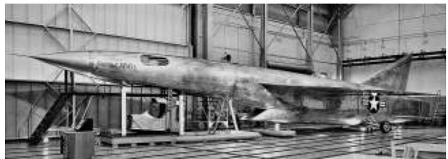
**Above and below: Two views of the full-size mockup of the XF-103. The upper picture shows the escape capsule which formed an elevator for crew access, located on the ground beneath the faired windscreen**
