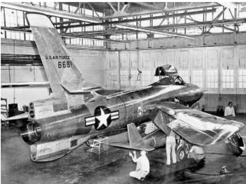
Left: The second prototype, 46-681, undergoing maintenance, and like the photo above, also configured for the XLR27 rocket engine. The four rocket pipes can easily be seen above and below the jetpipe. The main-wheel undercarriage doors located close to the wing tip are easily visible in this view
