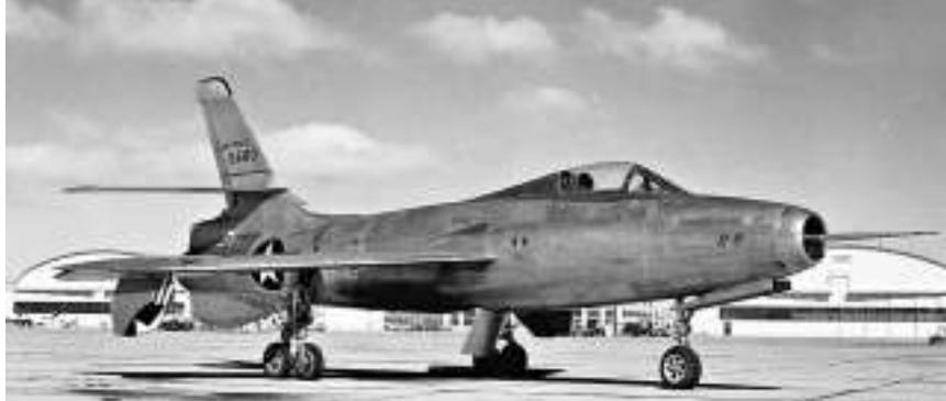
**Above: Prototype XF-91 46-680 with its original nose intake and a conventional tail fitted. The tandem mainwheels are clearly apparent in this view. Below: Second prototype XF-91 46-681, fitted with a nose radome, conventional tail, and carrying two 541 US gallon underwing fuel tanks**
