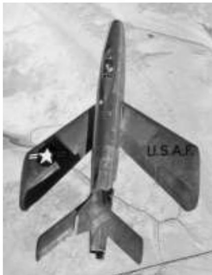
**Above: This view of the second prototype XF-91 shows the planform of the wings to good effect. The widest part of the wing chord can be seen to be nearest to the tips**
